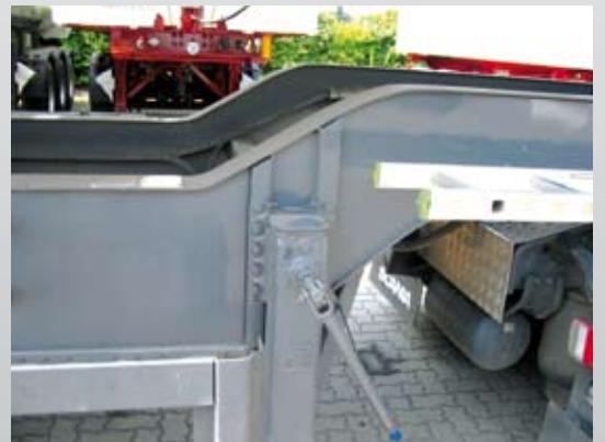
Offset chassis for reduced total height
