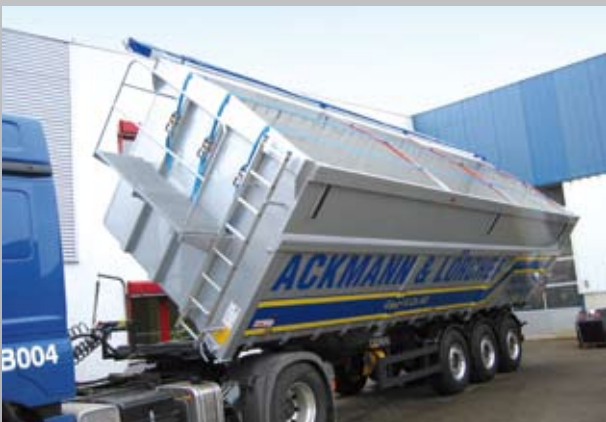
2-way tipper semitrailer with split sidewalls
