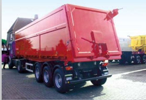
Top-hinged tailgate with grain hatch
