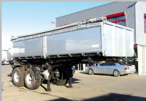
2-axle 3-way tipper semitrailer
