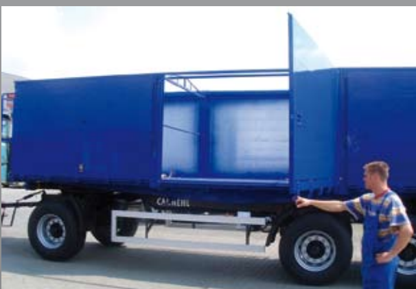
3-way tipper trailer with lateral wing gate
