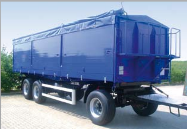
3-way tipper trailer with lateral wing gate
