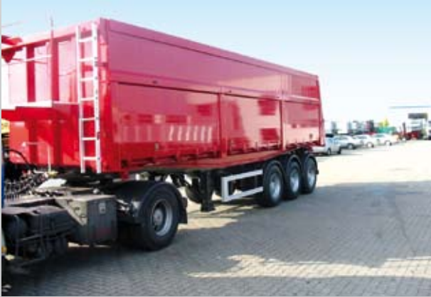
2-way tipper semitrailer with split sidewalls
