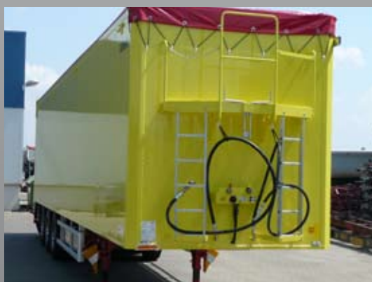
Platform with access from both sides
