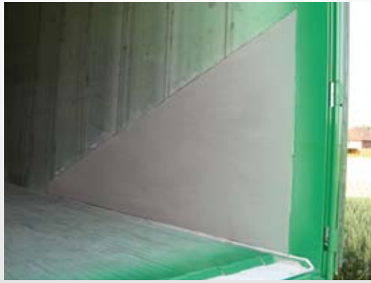
Wear panel on sidewall
